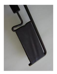
The membrane is the sensor of the **OILSPY** hydrocarbons detector.
