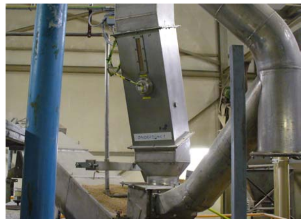
Sensor HUMY3000 with fitting for a continuous measurement in grain material flow
