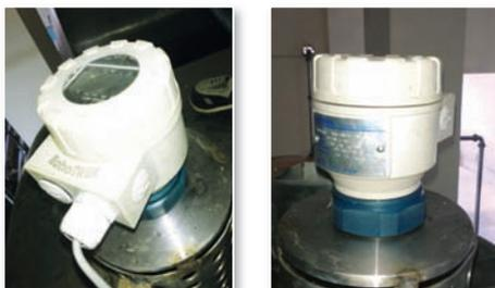
In this second case the devices are equipped with sensor filled with food industry compatible oil (as pressure transmitting medium) and DIN 11851 pipe coupling or Tri-Clamp sanitary process connection. But still as the density of the milk varies batch to batch there can be effect on the accuracy of these transmitters. Also the cost of needed regular
